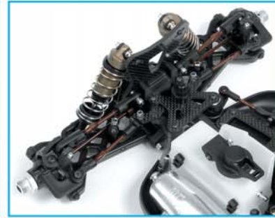
New narrow servo saver and steering system with ultra short graphite steering plate
