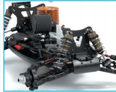
All new suspension geometry features Zero King-pin suspension concept
